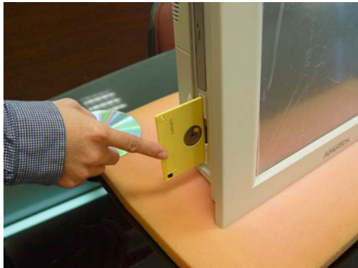
Figure 3.1: Inserting and ejecting a floppy disk
